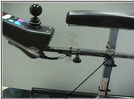
Attach cable to controller support and armrest stem
