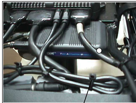
Coil the excess controller cable and hold in position with cable ties.
